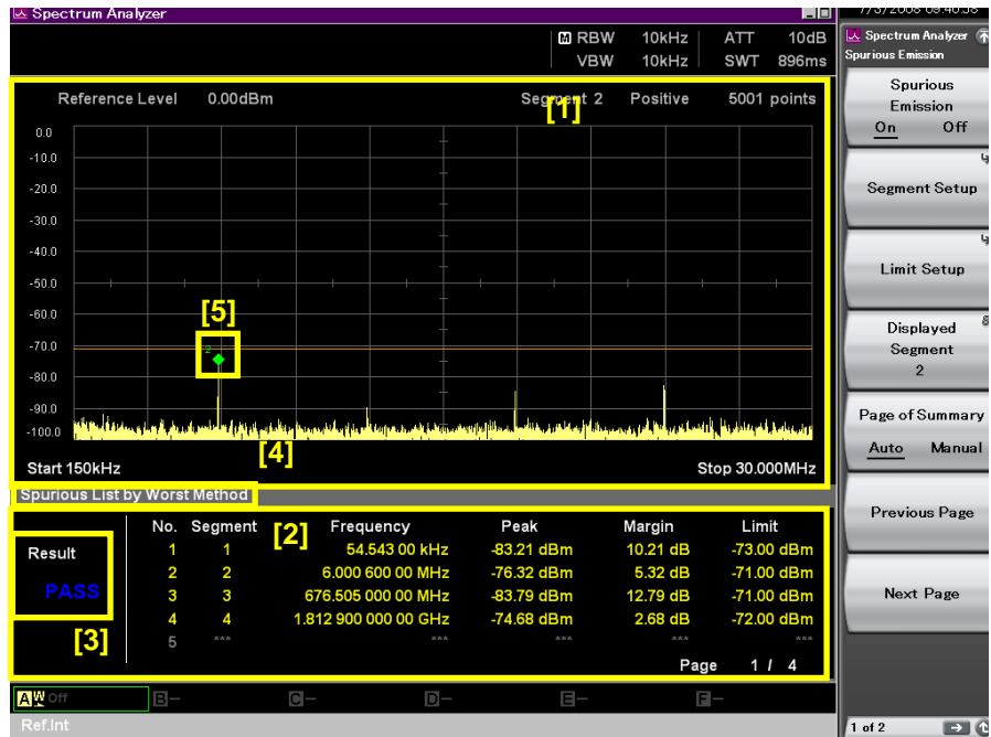
Figure 7.7-8 Display items of Spurious Emission measurement result (When Result Type is set to Worst.)
